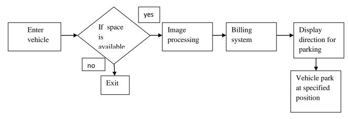
The Smart Parking System is designed to allow driver approaching a parking area to make an informed decision on where to park long before they arrive at each critical decision making point. Using efficient traffic and safety engineering, Intelligent Parking then guide the driver to these open bays with minimum attempt in the least time possible.
